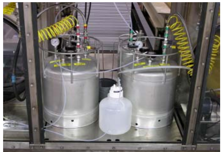
These reactors are a part of the chemical agent transfer system (CHATS) used for Operation Swift Solution. They mix the chemical agents with caustic materials to make hydrolysate.
